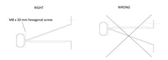
2. Attach the tubes to the wall. Adjust the foot so that the distance between the fixing screws is approximately 150 mm, or more, if necessary.
