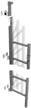
4. Principle drawing of the launching of the ladder
