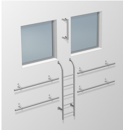
2. Escape route between two windows
