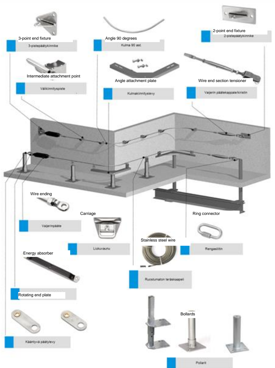
2. Parts of the system (in particular when attached to the wall and bollards).
